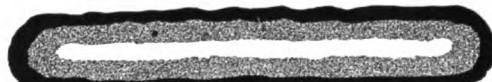
Partial impregnation—one stage in the effort to attain complete impregnation—discarded by us when the result shown below was accomplished.
